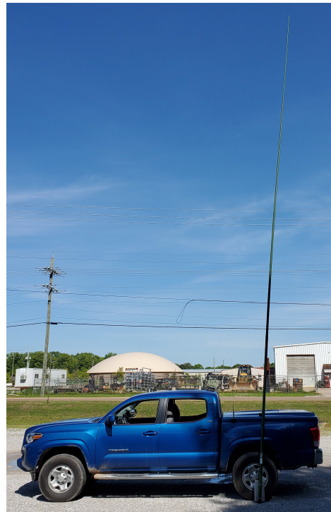
(b) MFJ-1912 supporting an MFJ-1916 mast
