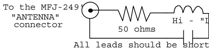
Tune the MFJ-209's frequency until the "SWR" meter reaches the lowest SWR. This is the resonant frequency of the load.
