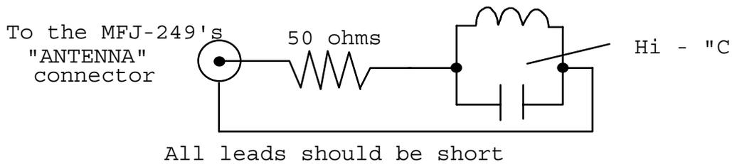
For high inductance values a series LC circuit should be used to measure resonant frequency. The inductor and capacitor should be connected in series through a 50Ω low inductance carbon resistor across the "ANTENNA" connector on the MFJ-209.
