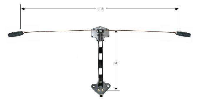
For best performance the antenna should be out in free space as much as possible. Do not allow any of the copper wire to touch any trees, etc. The ladder line should be at least 6" away from anything conductive. DO NOT TAPE LADDERLINE TO THE LEG OF A TOWER.
