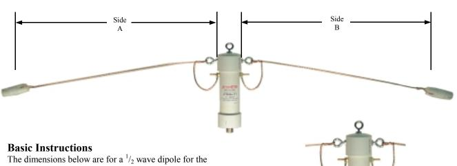
The dimensions below are for a  $^{1}/_{2}$  wave dipole for the ham bands just to get you started. These are starting dimensions. Size of wire, environment, etc can change the length of wire needed. It is always best to cut your wire a little long. Then when tuning just fold the wire back on itself so you can lengthen it later.
