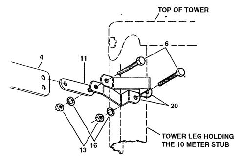
Figure 5 Installation to Tower Leg
