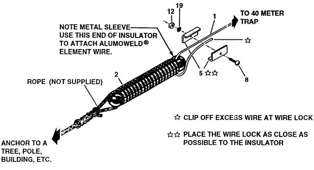
Figure 4 Antenna Wire to Insulator
