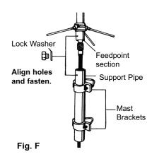
7. Attach assembled antenna on mast, taking balance into account.
