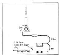
\* Using fuse greater than 0.5 Amp may cause damage to mount.
