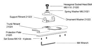
• Installing Motor Drive to Bracket
