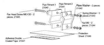
• Installing Motor Drive to Bracket
