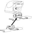
\* If proper angle adjustment is not possible due to contact between the mount bracket and the car body, move installation to different location while maintaining proper raise/lower direction.
