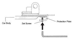
• Proper angle adjustment on trunk/hatchback installations:
