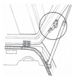
Install the bracket on hatchback as shown in the above figure with set screws and small hexagonal wrench. To avoid damaging the car body, insert protection plate into the place where set screws and the body contact.
