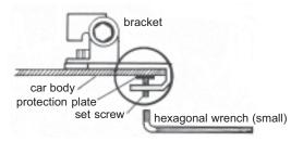
Use set screws attached to install the bracket.
