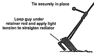
FIG-12B: Tying Off Guys to Anchor Stakes
