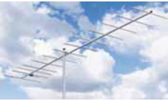
across the entire 2 meter band. New and experienced hams will enjoy 15.8 dBi gain on FM, packet, CW, or sideband across the 4 MHz operating range. The A13B2 is easily mounted vertically or horizontally for maximum performance on your favorite mode. Its optimum boom length makes it a popular antenna that fits just about anywhere. The new UltraMatch balanced feed on the A13B2 provides a 50 Ohm match via a standard SO-239 UHF female connector.
