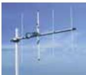
**26B2** This antenna offers the highest gain of any 2 meter FM antenna in the world. The A26B2 includes 2 complete A-13B2 antennas, stacking boom and phasing harness. Frequency range 144-148 mhz, 26 elements, 17 dbi of gain, longest element 39.75 in, boom length 15ft, max power 1500W, 21.5 lbs
