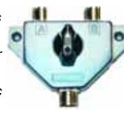
**MFJ1702C** 2-position coax switch has a new center ground protection! Better than 60 dB isolation at 300 MHz and better than 50 dB at 450MHz. 50 Ohm. Unused terminal is automatically grounded for static and RF protection. It has less than 0.2 dB
