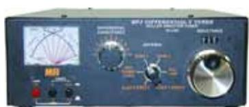
and easier than ever. It ends constant re-tuning with broadband coverage and gives you minimum SWR at only one best setting. 1.5kW PEP. 1.8-30 Mhz. Roller inductor makes tuning smooth and easy. Turns counter lets you quickly re-tune to frequency. Lighted cross-needle meter reads SWR/forward/reflected/peak/average power in 2 ranges. Current balun reduces feedline radiation and forces equal currents into unbalanced antennas.
