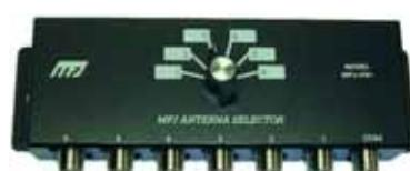
automatically grounded. Quality SO-239 connectors for hookup to your antennas. Handles 2kW PEP SSB, 1kW CW. 50 - 75 Ohm loads. Measures a compact 10" W x 3" H x 1" D.
