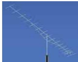
**224WB** This 222MHz 4 element beam is perfect for Packet, FM repeaters, or sideband/CW. It can be mounted for vertical or horizontal polarization. Forward gain of 10.2 dbi, Boom length 3 ft, Longest element 26.7 inches, Mast size 1.25-2", Wind Load .23 ft2, 9.9 lbs
