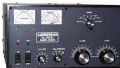
**AL800H** Output power: 1250 watts PEP, single 3CX800A7; 1500 watts plus, two 3CX800A7s All band operation: 160-15 meters including WARC bands. User modifiable for 12 and 10 meters. Genuine Eimac tube(s): Model AL-800 has single Eimac 3CX800A7; Model AL-800H has two Eimac 3CX800A7s
