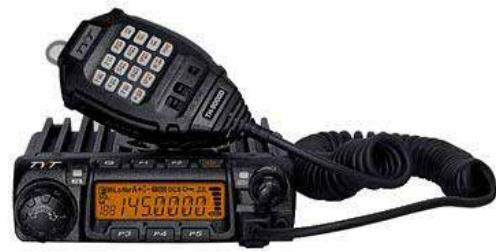
Lock-Out Channel name editing Reverse frequency Talk around Voice prompt Time-out Timer Auto Power off VFO step setting:5/6.25/10/12.5/20/25/50kHz 200 memory channels FM radio CTCSS/DCS DTMF/2 Tone coder
