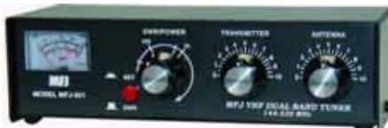
**MFJ921** The MFJ-921 Dual Band VHF Antenna Tuner covers 2 Meters and 220 MHz. Its built-in SWR/Wattmeter measures SWR in 2 power ranges – 300 or 30 Watts. The meter is usable for both 144 MHz and 220 MHz bands. It will give you low SWR with practically any antenna. The MFJ-921 is designed to match a wide range of impedances for both mobile/base operation. It will handle up to 200 Watts of output power. The antenna tuner has SO-239 input/output connectors, wing nut post ground.
