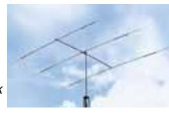
**A4496S** Use one of these 440MHz beams for your FMPacket needs. Both work great for vertical/horizontal polarization. 6 elements, 10.5 dbi of gain
