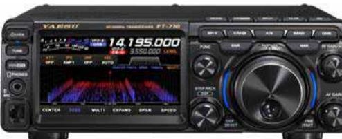
**FT710** Includes Yaesu SP-40 external speaker YAESU is excited to announce a new HF/50MHz 100W SDR Transceiver - FT-710 AEES. The new FT-710 AEES is a compact design yet provides 100W output, utilizing the advanced digital RF technology introduced in the FTDX101 and FTDX10 series.
