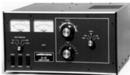
**AL82** The Ameritron AL-82 Linear Amplifier is designed to give you years of trouble free service at the full legal output power limit. An 1800 watt continuous commercial rated Hypersil transformer is standard with heavy duty rectifiers in a full wave bridge supply with computer grade capacitors. Two bias settings allow either high efficiency RTTY and CW operation at 1500 watts of output at nearly 70% plate efficiency or low distortion 1500 watts PEP, SSB or SSTV output.
