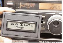
MFJ AutoTrak™ automatically locks on, tracks and displays CW to 99 WPM.
