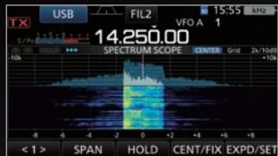
DPD OFF (Signal Received on the IC-7300)
