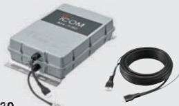
AH-730 Covers 1.8 ~ 54 MHz with a 7 m, 23 ft or longer wire antenna. Max. input: 150 W PEP, 100 W continuous. Controller cable (10 m, 32.8 ft) is supplied with the AH-730.
