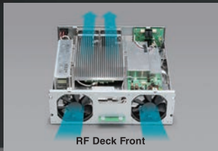
Effective Cooling System with Four Fans
